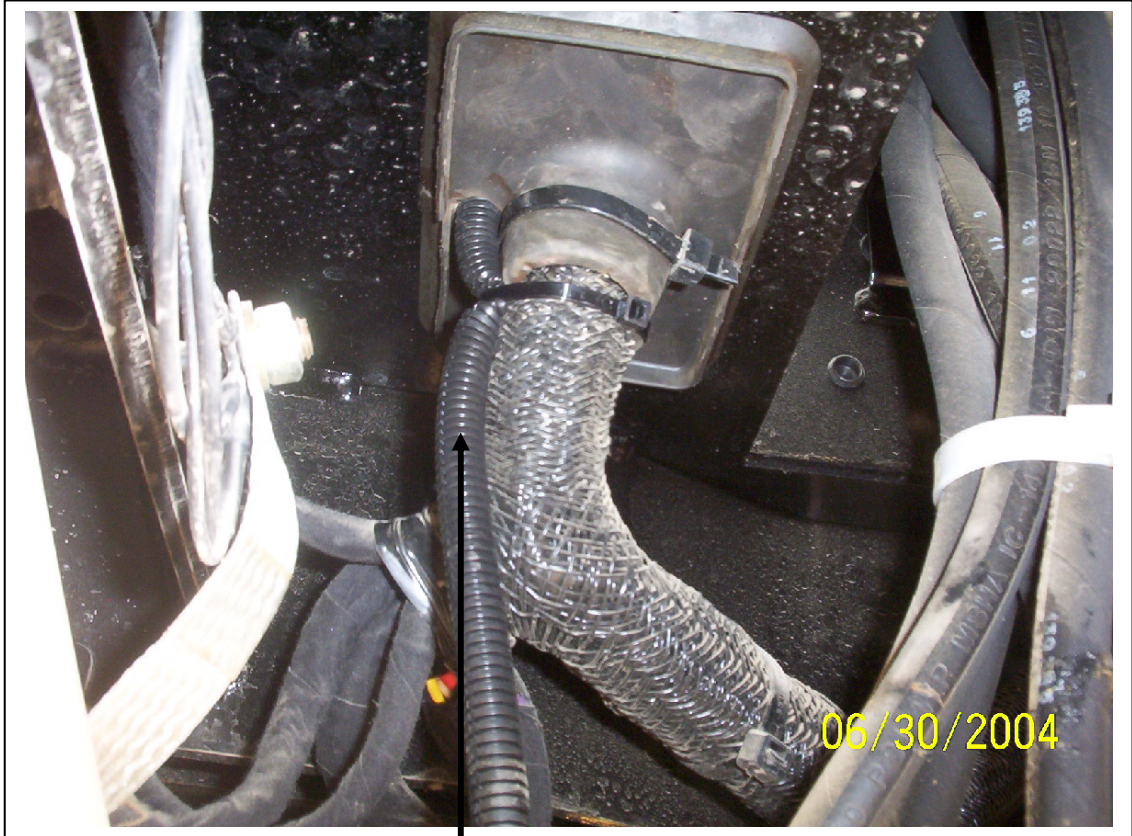
Clutch wire entering the cab on the right side of cab below the electrical access panel inside right cab door. Connect it to the thermostat.
