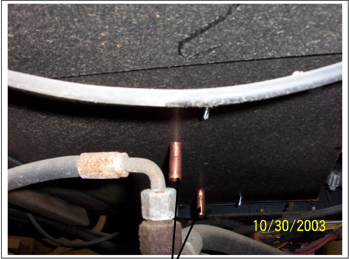
Copper drain tubes seen from under the cab. Install plastic tube and restrictors onto these tubes.
