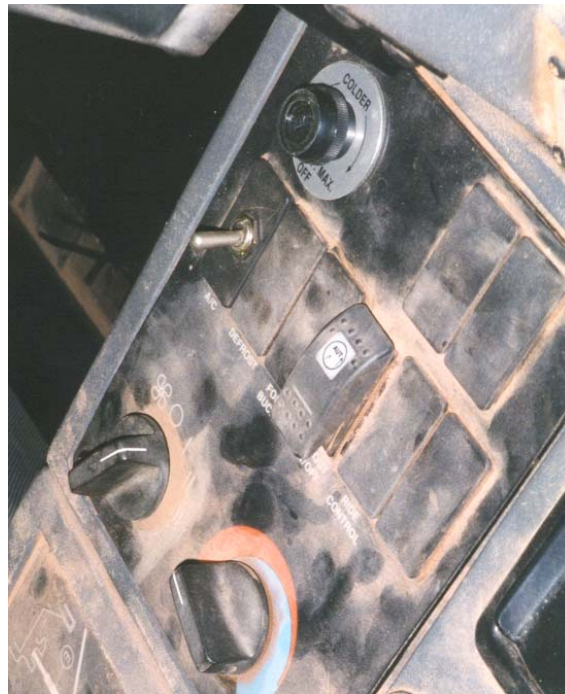
Thermostat location on panel. (older machine)
